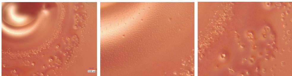
(a) Phase explosion damage
