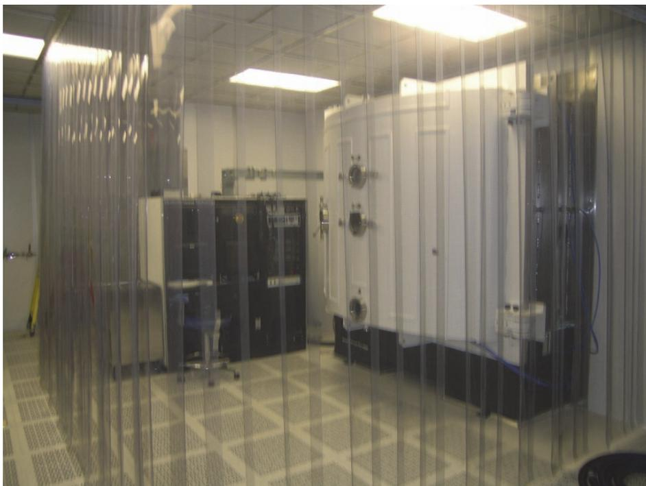
Fig. 1. The Sandia large optics coating chamber and process control console.
